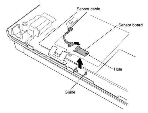
Figure 4-43 Removing the sensor board
